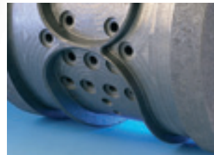
Ceratzit blanks are mounted on steel shafts (contracted) and ground sharply. Two contra-rotating rolls cut millions of diapers a day from the wadding.
