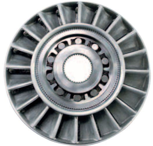
One-way clutch inner race and Cam for a torque converter one-way clutch. The clutch is installed in the aluminium stator.
