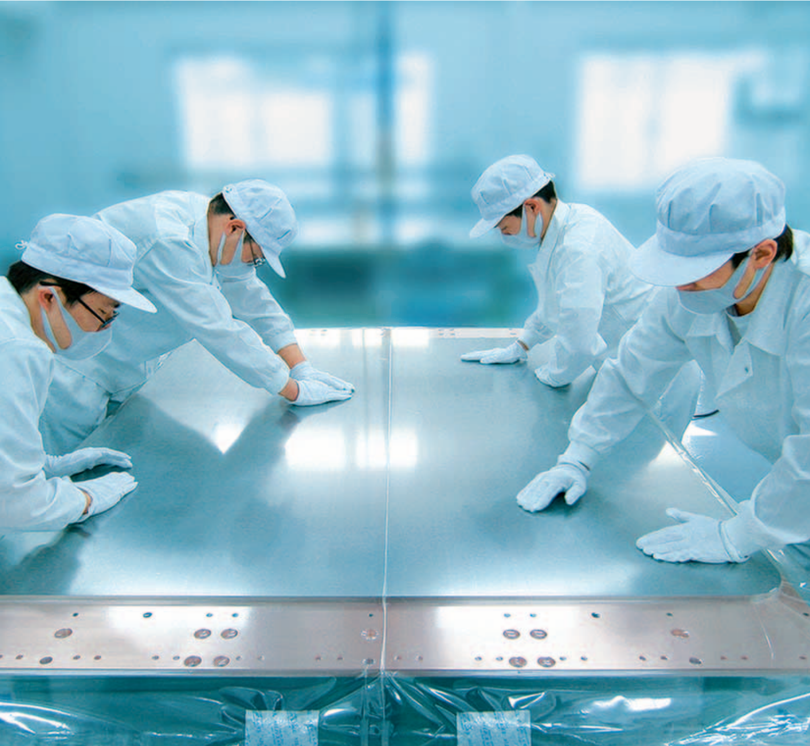
Finishing and packaging of bonded sputter targets in our bonding shop in Japan
